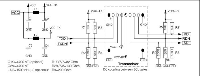
\*Recommended choke is Siemens Matsushita B78108-S1153-K or B78148-S1153-K (Q<sub>min</sub>=60, max. DC resistance=0.6 Ohm).
