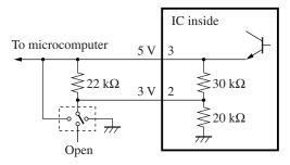
4) The Reset output becomes Low (0.15 V or less) by pin 3 voltage (at  $V_3 \le 4.1$  V).
