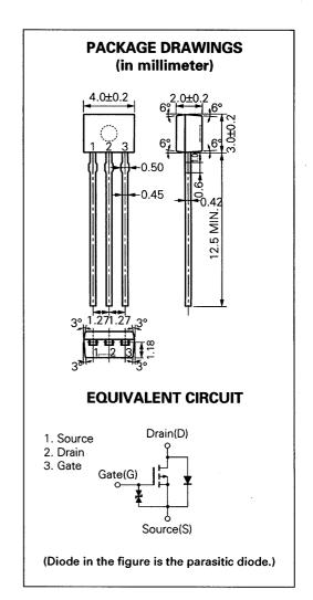
The diode connected between the gate and source of the transistor serves as a protector against ESD. When this device is actually used, an additional protection circuit is externally required if a voltage exceeding the rated voltage may be applied to this device.
