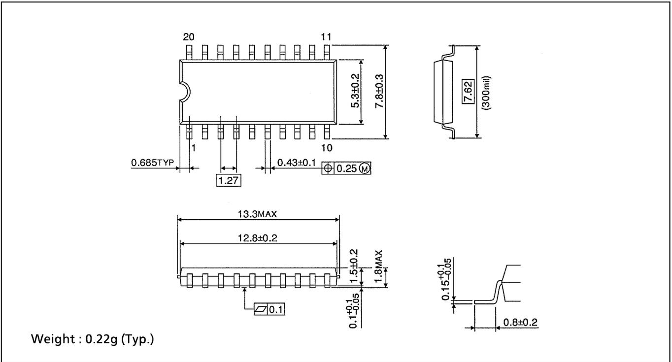
**SOP 20PIN (300mil BODY) PACKAGE DIMENSIONS (SOP20-P-300-1.27)**
