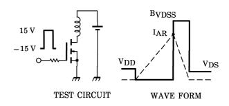
$$\begin{array}{l} \text{Peak I}_{AR} = 30 \, \text{A, R}_{G} = 25 \, \Omega \\ \text{V}_{DD} = 50 \, \text{V, L} = 1.66 \, \text{mH} \end{array} \quad \text{E}_{AS} = \ \frac{1}{2} \cdot \text{L} \cdot \text{I}^{2} \cdot \ ( \ \frac{\text{BVDSS}}{\text{BVDSS} - \text{V}_{DD}} \ ) \end{array}$$
