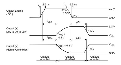
Figure 3  $t_{pLZ}, t_{pHZ}, t_{pZL}, t_{pZH}$
