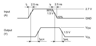
Figure 2 t<sub>pLH</sub>, t<sub>pHL</sub>
