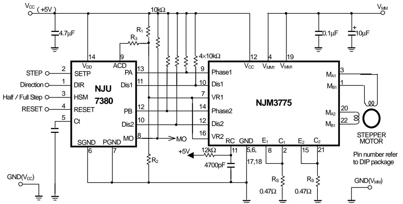
Fig.3 Typical stepper motor driver application with NJM3775.
