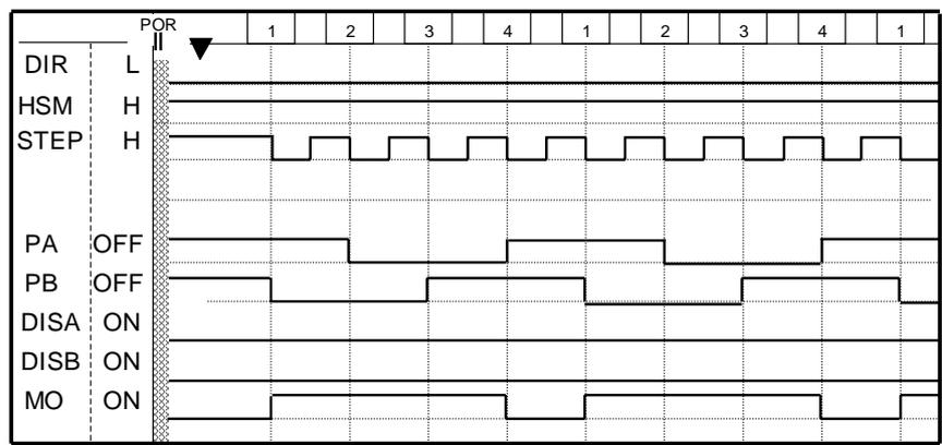
Fig.5-3 Half-step mode,forward
