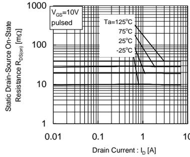
Fig.2 Static Drain-Source On-State Resistance vs. Drain Current (1)
