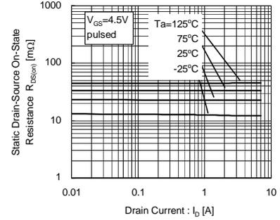
Fig.3 Static Drain-Source On-State Resistance vs. Drain Current (2)
