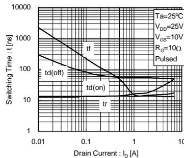
Fig.8 Switching Characteristics
