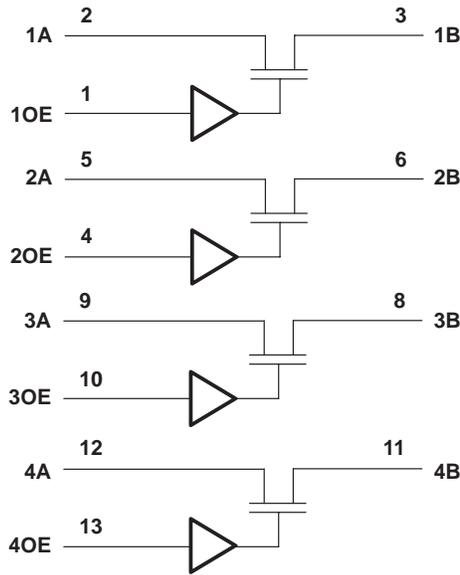
Pin numbers shown are for the D, DB, DGV, and PW packages.
