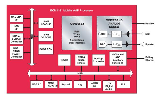
The BCM1161 VoIP processor offers a high level of system integration, performance, and features for wireless IP phone handsets. The chip architecture was designed specifically with low-power and small footprint in mind for wireless handheld applications.
