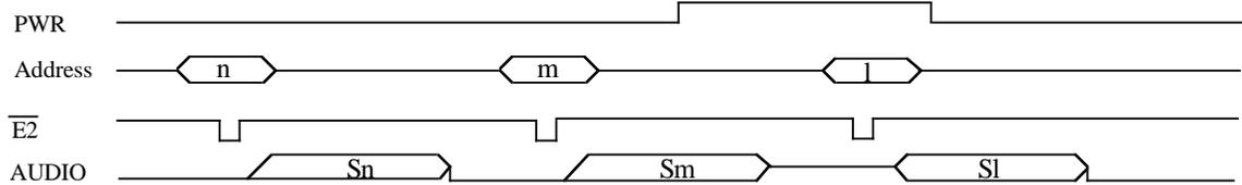
**X. Mask as Retrigger / CPU mode ( 6 - bit address )**
