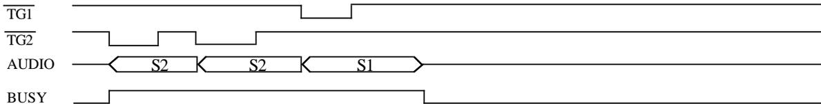
**V. 4. Retrigger function , Trigger Mask = Edge or Level, Overlap trigger inputs**
