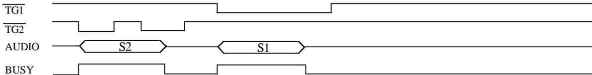
**IV. 2. Stand Alone mode, No Retrigger function, Level Trigger Mask, low active, two non - overlap trigger inputs**
