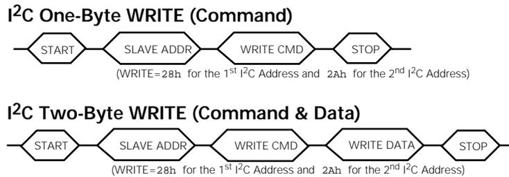
**NOTE:** The Status Register RDY bit must be read and checked prior to the START condition of either WRITE sequence above. Refer to the One Byte READ (Status Only) in [Figure 5](#) for more information on reading the Status Register.
