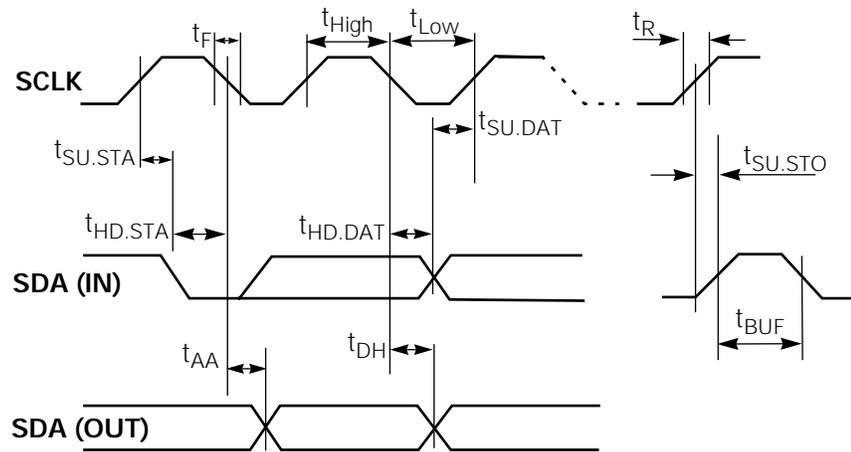
TABLE 6. I<sup>2</sup>C SERIAL TIMING MIN/MAX
