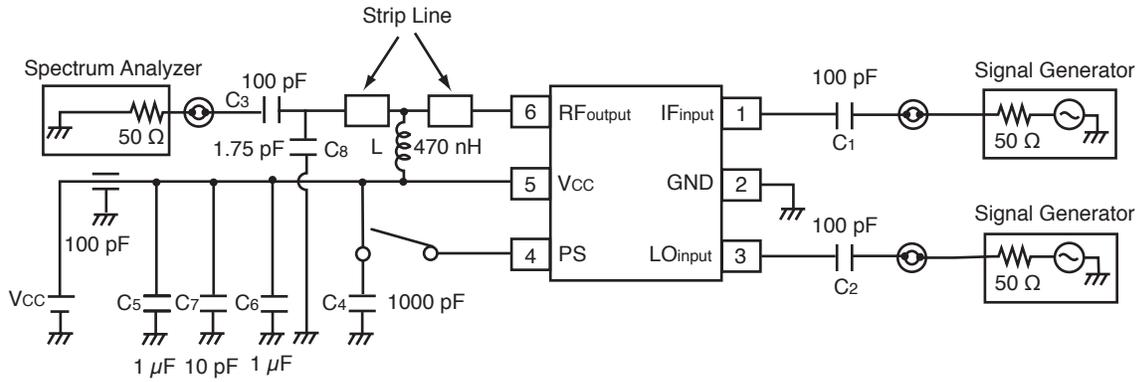
**EXAMPLE OF TEST CIRCUIT 3 ASSEMBLED ON EVALUATION BOARD**
