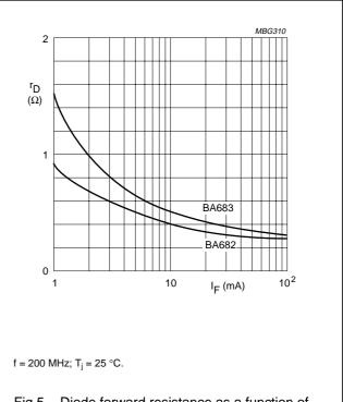
Fig.5 Diode forward resistance as a function of forward current; typical values.
