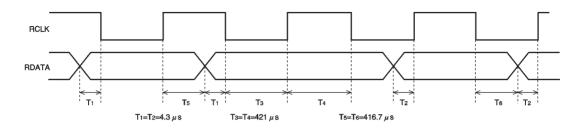
The clock (RCLK) frequency is 1187.5Hz. Depending on the state of the internal PLL clock, the data (RDATA) is replaced in synchronous with either the rising or falling edge of the clock. To read the data, you may choose either the rising or falling edge of the clock as the reference. The data is valid for 416.7 µs. after the reference clock edge.
