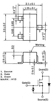
(Diode in the figure is the parasitic diode.)
