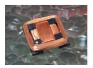
The 3DC series of surface mountable 3D antenna inductors is the very first of its type specifically designed for 125kHz transponder applications. The coil dimensions are optimised to achieve maximum sensitivity on each coil axis.
