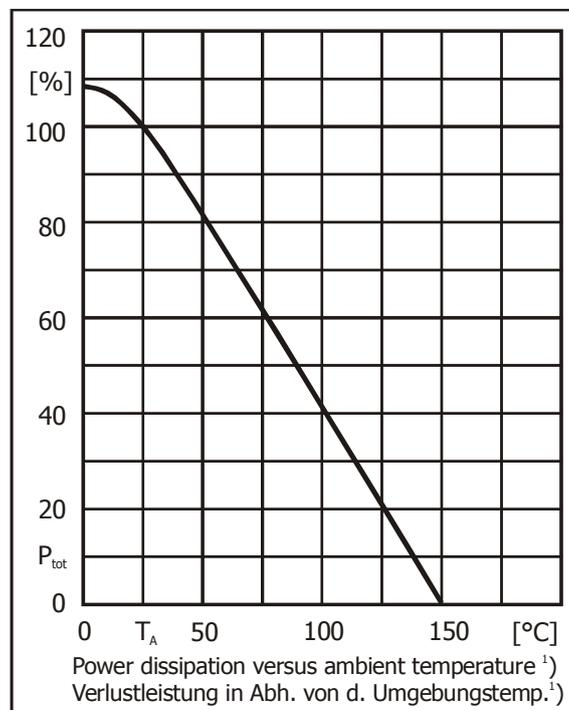
1 Mounted on P.C. board with 3 mm<sup>2</sup> copper pad at each terminal
