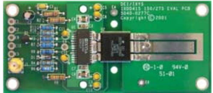
Figure 1 - EVDD415 Evaluation Board DEI DE275-102N06A Device Installed In Low-Power Configuration For Illustration Purposes Only
