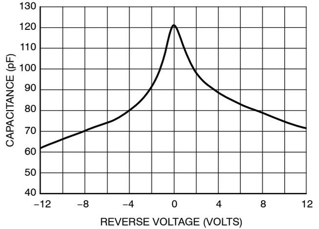
Figure 4. Typical Line Capacitance vs. Reverse Bias Voltage
