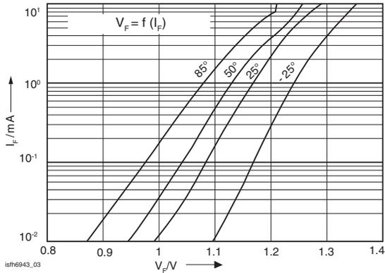
Figure 3. LED Current vs. LED Voltage
