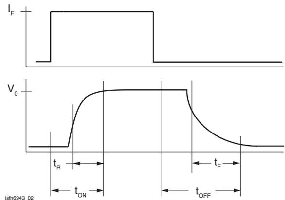
Figure 2. Switching Waveform
