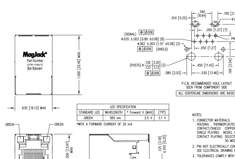
1. CONNECTOR MATERIALS: HOUSING: THERMOPLASTIC UL94 V-0 CONTACT/SHIELD: COPPER ALLOY SHIELD PLATING: NICKEL OR TIN CONTACT PLATING: SELECTIVE GOLD. 50 MICRO-INCHES MIN. IN CONTACT AREA.
