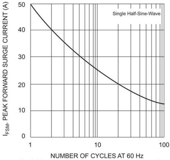
Fig. 3 Max Non-Repetitive Peak Forward Surge Current
