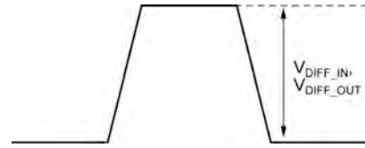
Figure 5b. Differential Voltage Swing
