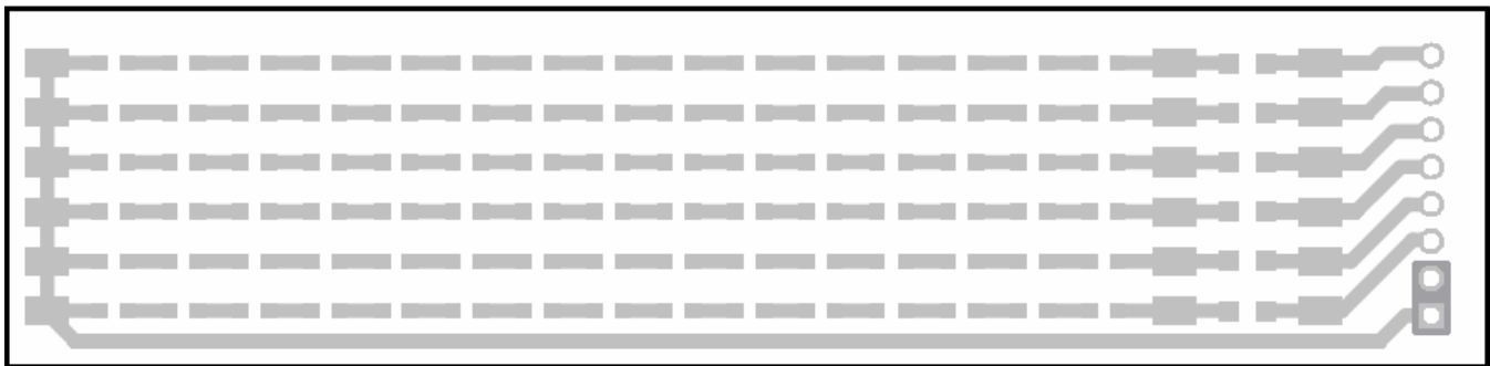
Figure 2—LED Board Top Layer
