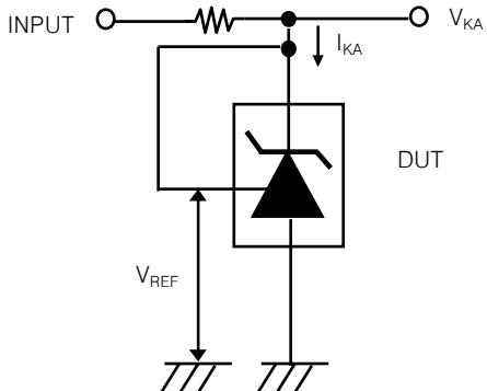
Fig. 2 Test Circuit for  $V_{KA} \geq V_{REF}$
