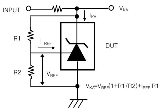
Fig. 3 Test Circuit for  $I_{KA(OFF)}$
