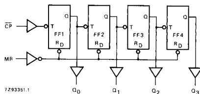
Fig. 6 Logic diagram (one counter).
