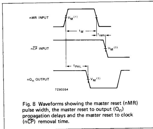
Fig. 8 Waveforms showing the master reset (nMR) pulse width, the master reset to output ( $Q_n$ ) propagation delays and the master reset to clock ( $n\overline{CP}$ ) removal time.
