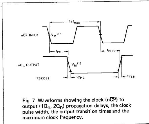
Fig. 7 Waveforms showing the clock ( $n\overline{CP}$ ) to output ( $1Q_n$ ,  $2Q_n$ ) propagation delays, the clock pulse width, the output transition times and the maximum clock frequency.
