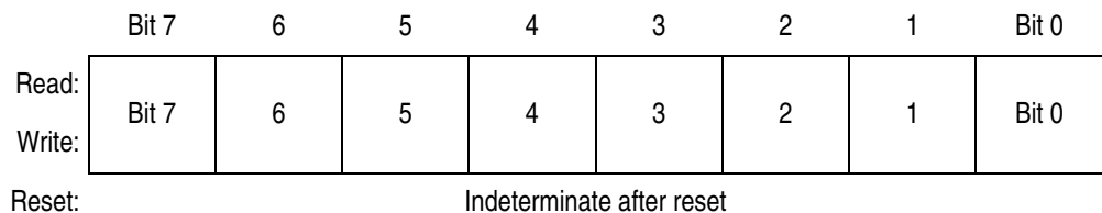
Figure 11-15. TIM Channel 1 Register Low (TCH1L)
