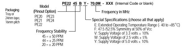
Consult factory for available frequencies and specs. Not all options available for all frequencies. A special part number may be assigned. Frequency Stability is inclusive of frequency shifts due to calibration, temperature, supply voltage, shock, vibration and load
