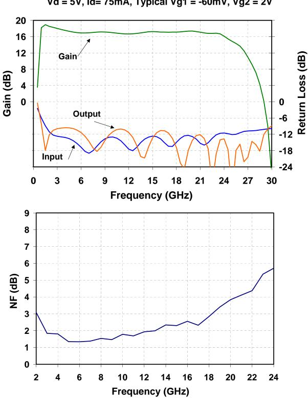
Vd = 5V, Id= 75mA, Typical Vg1 = -60mV, Vg2 = 2V
