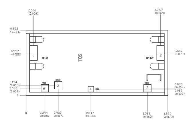
Units: millimeters (inches) Thickness: 0.100 (0.004) Chip edge to bond pad dimensions are shown to center of bond pad
