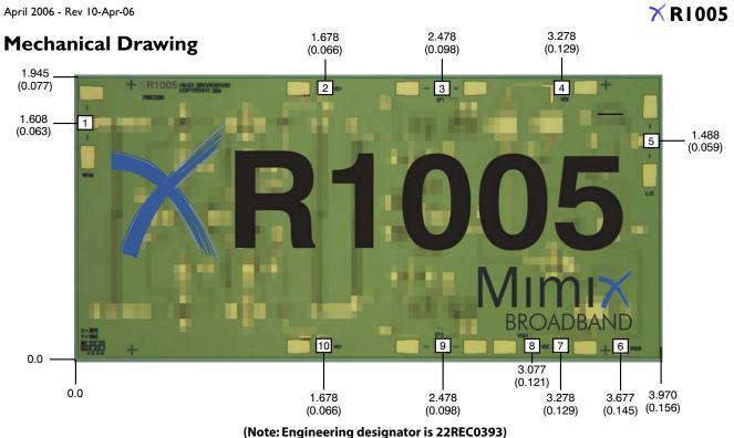
Units: millimeters (inches) Bond pad dimensions are shown to center of bond pad. Thickness: 0.110 + -0.010 (0.0043 + -0.0004), Backside is ground, Bond Pad/Backside Metallization: Gold All DC/IF Bond Pads are  $0.100 \times 0.100 (0.004 \times 0.004)$ . All RF Bond Pads are  $0.100 \times 0.200 (0.004 \times 0.008)$ . Bond pad centers are approximately 0.109 (0.004) from the edge of the chip. Dicing tolerance: +/-0.005 (+/-0.0002). Approximate weight: 4.787 mg.
