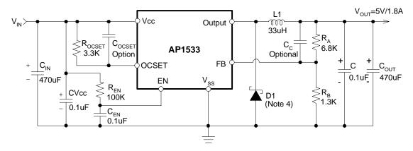
$$V_{OUT} = V_{FB} x (1+R_A/R_B)$$
