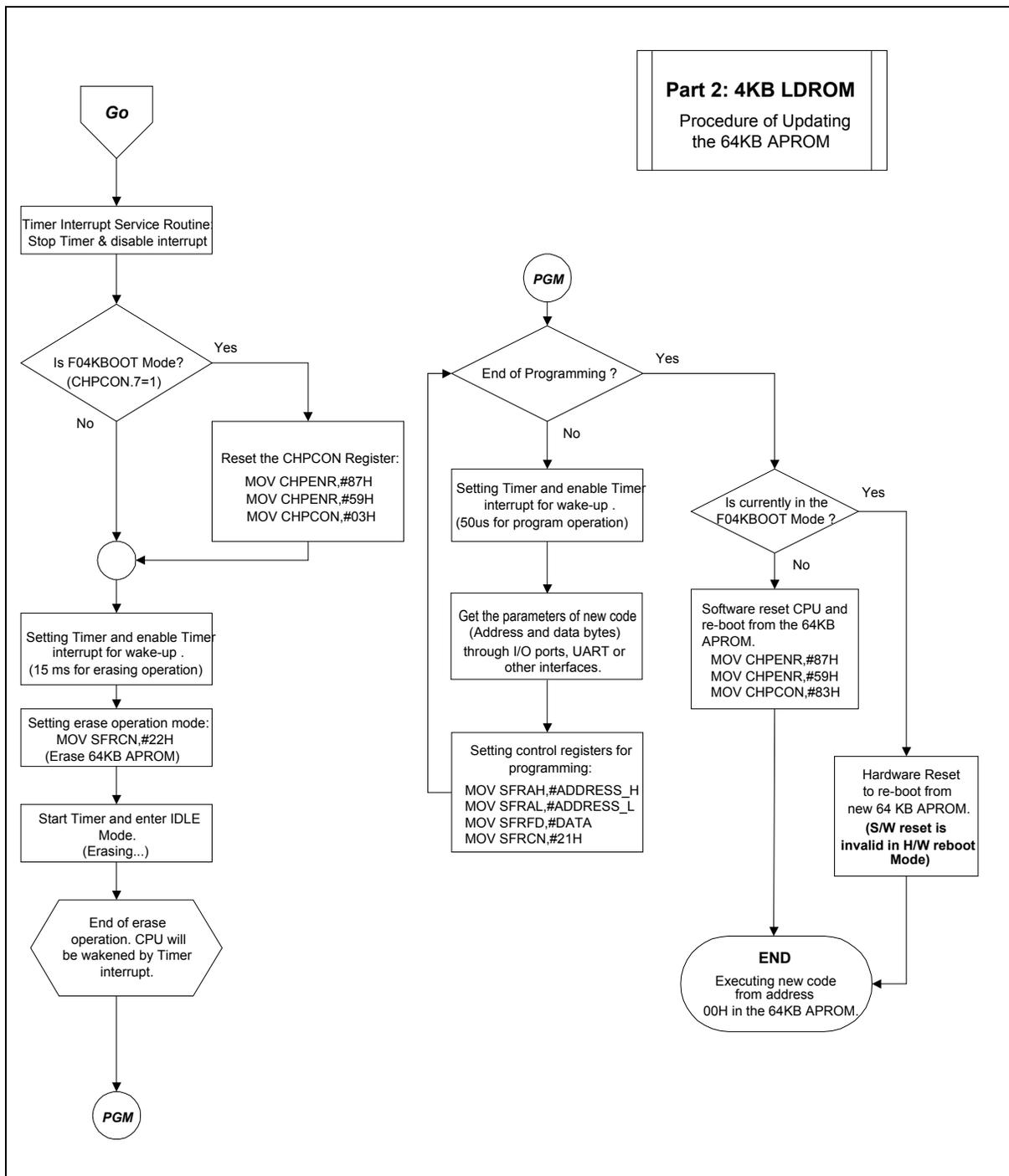
Figure 15-2 The algorithm of ISP for LD ROM
