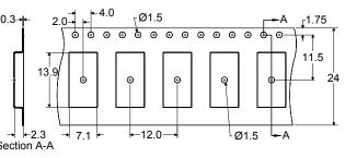
Dimensions shown are nominal in millimeters Packaging quantity: 2000 units/reel
