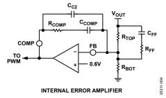
Figure 19. Compensation Using Feed-Forward
