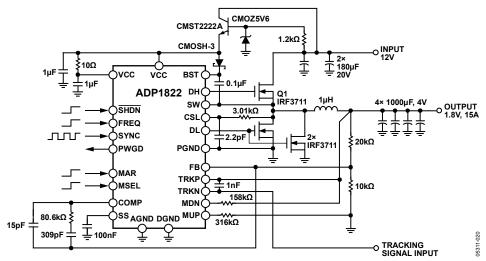
Figure 21. Typical Application Circuit, 12 V Input
