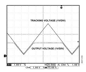
Figure 17. Output Voltage Tracking Response
