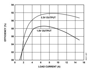
Figure 6. Efficiency vs. Load Current,  $V_{IN} = 12 \text{ V}$ ,  $V_{OUT} = 3.3 \text{ V}$ , 1.8 V
