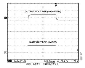
Figure 16. Output Voltage Margin-Up Response
