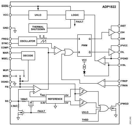
Figure 3. Simplified Block Diagram
