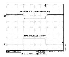
Figure 15. Output Voltage Margin-Down Response
