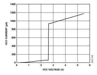
Figure 7. VCC Supply Current vs. Voltage
