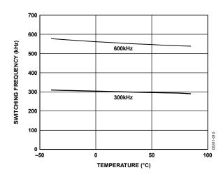
Figure 9. Switching Frequency vs. Temperature
