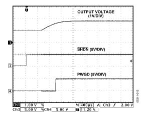
Figure 12. Power-On Response, Prebiased Output
