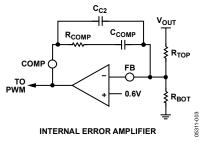
Figure 18. Compensation Using the ESR Zero
