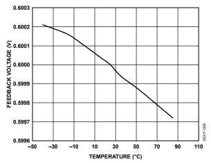
Figure 8. FB Regulation Voltage vs. Temperature
