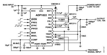
Figure 1. Typical Operating Circuit
