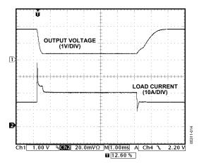
Figure 13. Output Short-Circuit Response and Recovery
