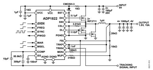
Figure 20. Typical Application Circuit, 5 V Input
