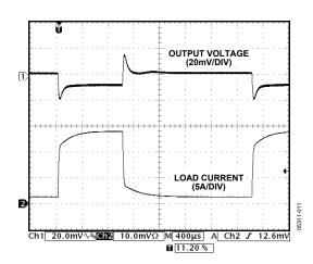
Figure 10. Load Transient Response, 1.5 A to 15 A
