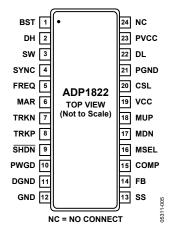
Figure 4. Pin Configuration
