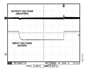
Figure 14. Line Transient Response, 10 V to 16 V
