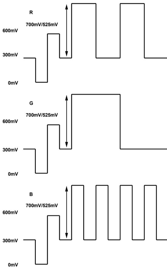
Figure 127. HD RGB Output Levels—RGB Sync Enabled
