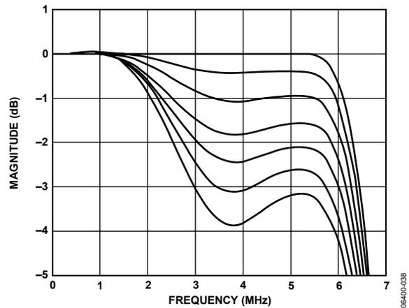
Figure 38. SD Luma SSAF Filter, Programmable Attenuation
