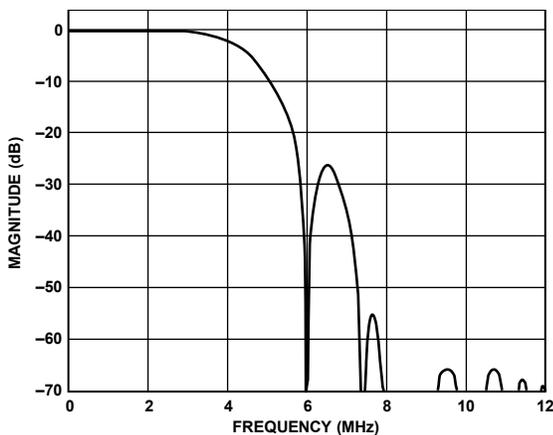
Figure 30. SD NTSC, Luma Low-Pass Filter Response
