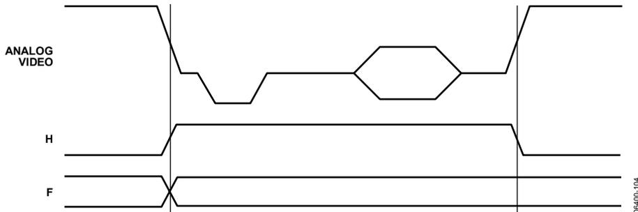
Figure 103. SD Master Mode 0, Data Transitions
