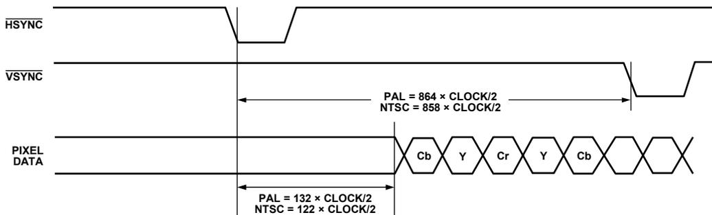
Figure 110. SD Timing Mode 2 Odd-to-Even Field Transition (Master/Slave)
