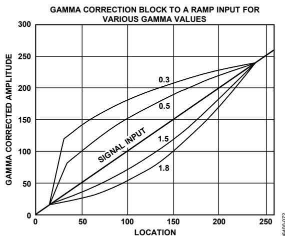
Figure 71. Signal Input (Ramp) and Selectable Output Curves
