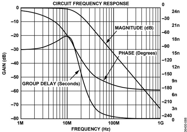
Figure 87. Output Filter Plot for SD, 16x Oversampling
