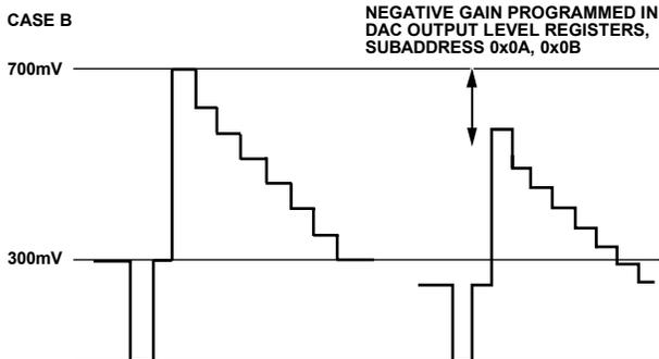
Figure 69. Programmable DAC Gain—Positive and Negative Gain
