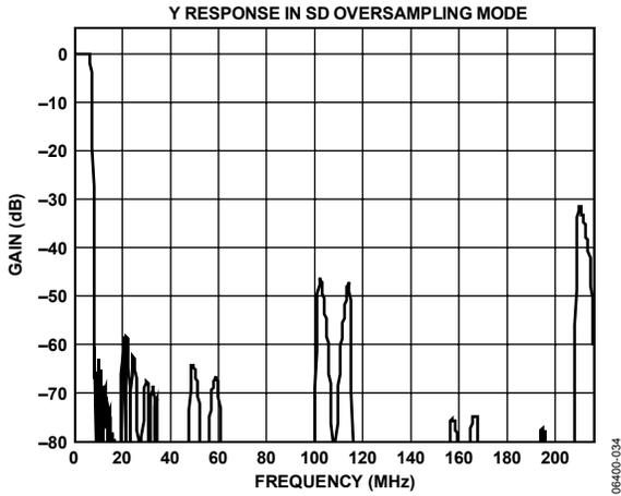
Figure 34. SD, 16x Oversampling, Y Filter Response
