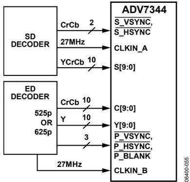
Figure 55. Simultaneous SD and ED Example Application
