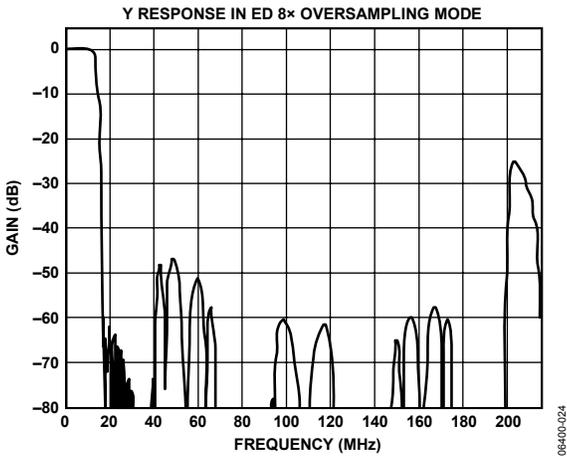
Figure 24. ED 8× Oversampling, Y Filter Response
