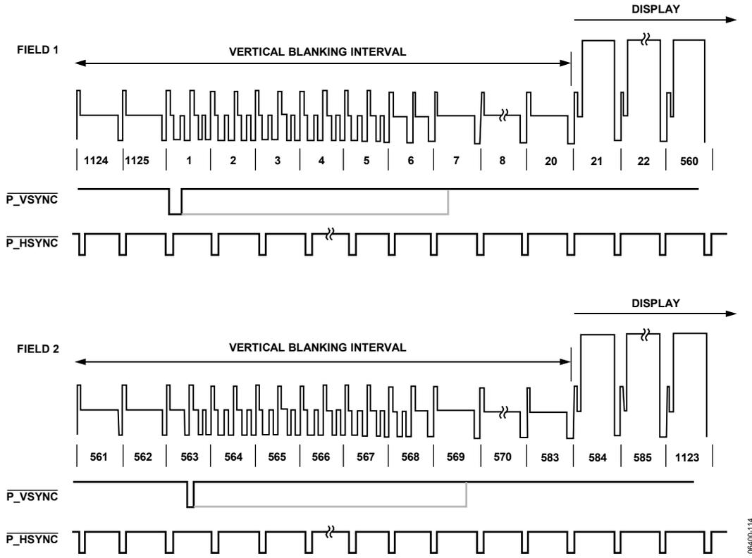
Figure 113. 1080i HSYNC and VSYNC Input Timing
