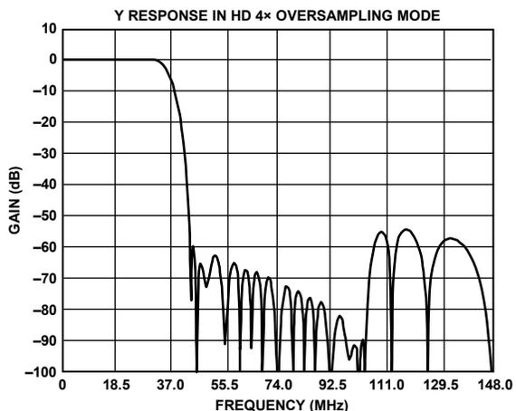
Figure 28. HD 4x Oversampling, Y Filter Response
