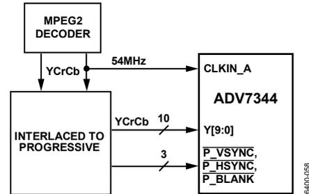
Figure 58. ED Only (at 54 MHz) Example Application
