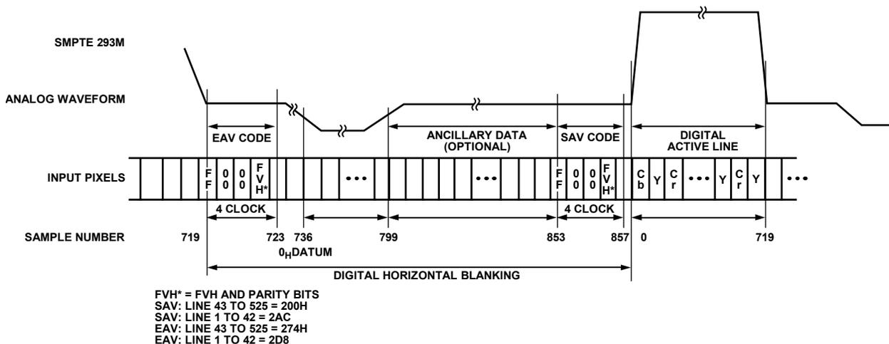
Figure 135. EAV/SAV Input Data Timing Diagram (SMPTE 293M)
