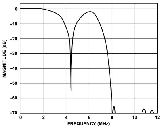
Figure 33. SD PAL, Luma Notch Filter Response
