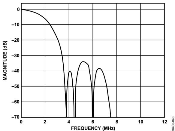
Figure 40. SD Luma QCIF Low-Pass Filter Response
