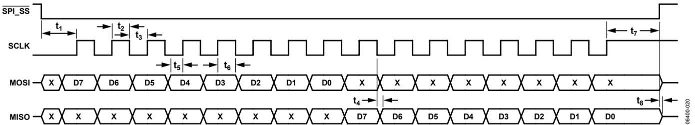
Figure 20. MPU Port Timing Diagram (SPI Mode)
