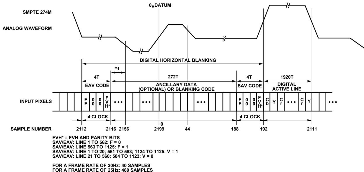
Figure 134. EAV/SAV Input Data Timing Diagram (SMPTE 274M)
