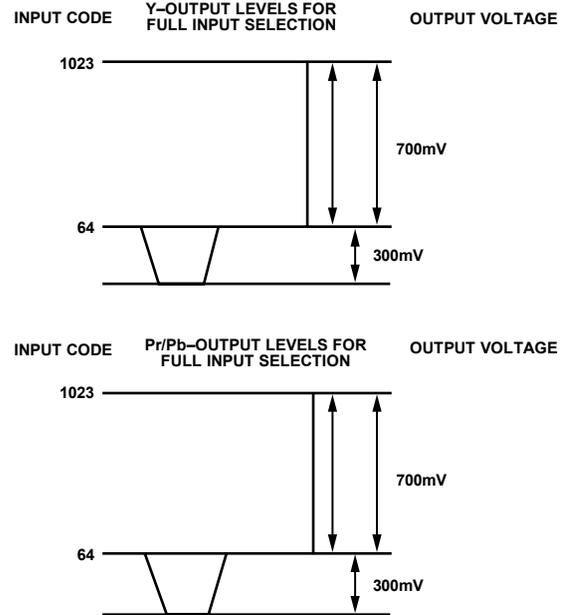
Figure 123. Output Levels for Full Input Selection
