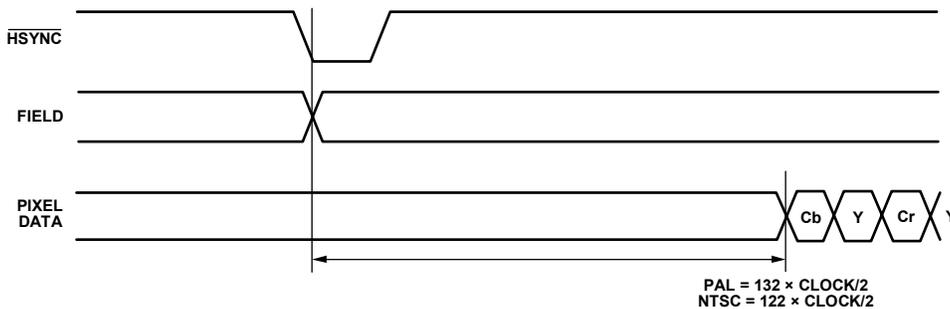
Figure 106. SD Timing Mode 1, Odd/Even Field Transitions (Master/Slave)
