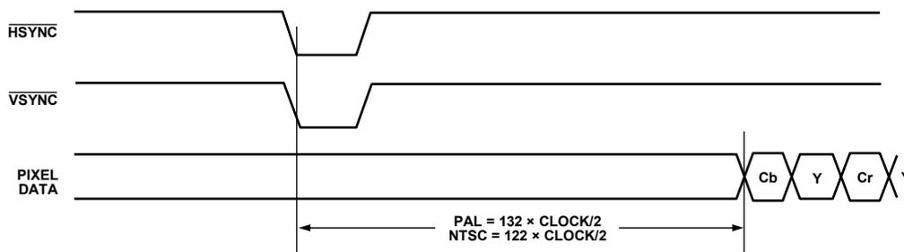
Figure 109. SD Timing Mode 2, Even-to-Odd Field Transition (Master/Slave)
