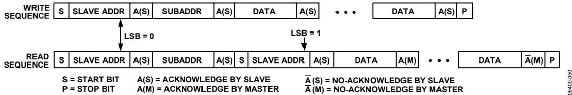
Figure 50. I<sup>2</sup>C Read and Write Sequence
