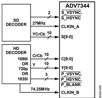
Figure 56. Simultaneous SD and HD Example Application
