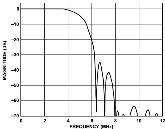
Figure 31. SD PAL, Luma Low-Pass Filter Response
