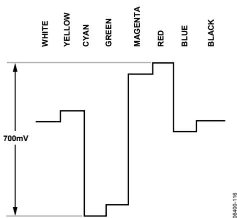
Figure 115. Pr Levels—NTSC
