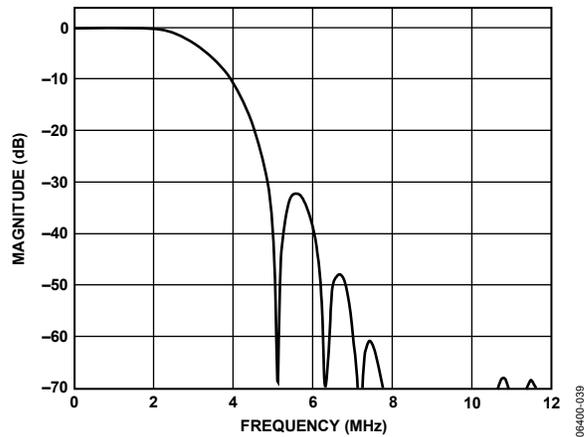
Figure 39. SD Luma CIF Low-Pass Filter Response
