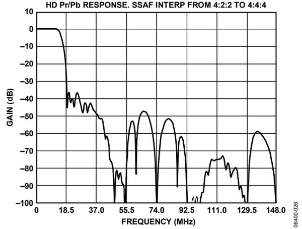
Figure 26. HD 4× Oversampling, PrPb (SSAF) Filter Response (4:2:2 Input)
