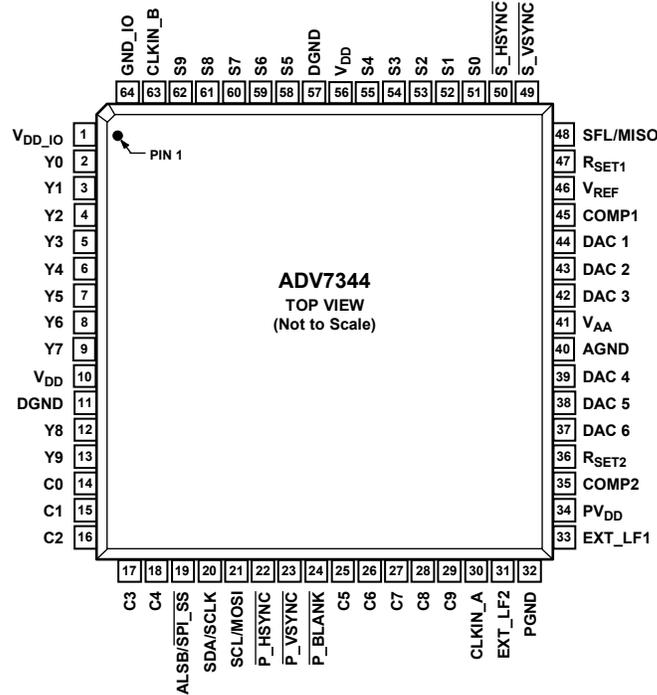
Figure 21. Pin Configuration
