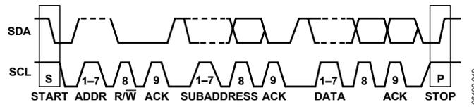
Figure 49. I<sup>2</sup>C Data Transfer
