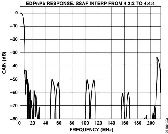
Figure 23. ED 8× Oversampling, PrPb Filter (SSAF) Response
