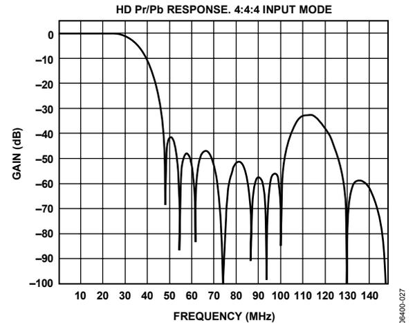
Figure 27. HD 4× Oversampling, PrPb (SSAF) Filter Response (4:4:4 Input)
