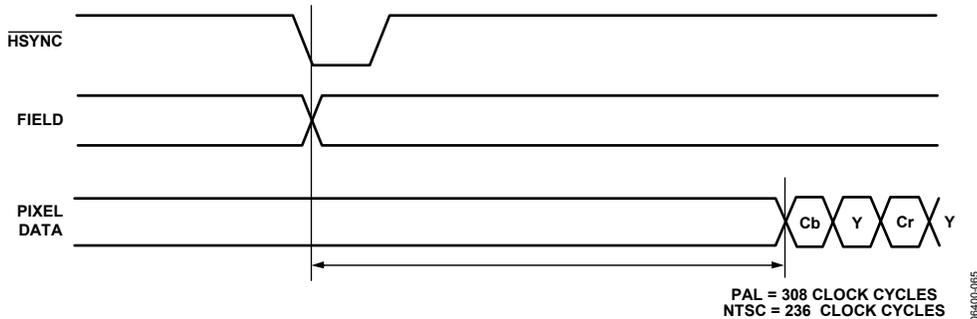
Figure 64. Square Pixel Mode Active Pixel Timing
