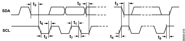
Figure 19. MPU Port Timing Diagram (I<sup>2</sup>C Mode)
