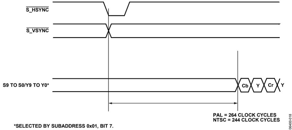
Figure 18. SD Input Timing Diagram (Timing Mode 1)
