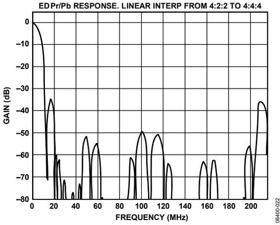
Figure 22. ED 8× Oversampling, PrPb Filter (Linear) Response
