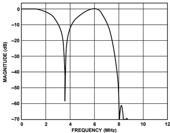
Figure 32. SD NTSC, Luma Notch Filter Response
