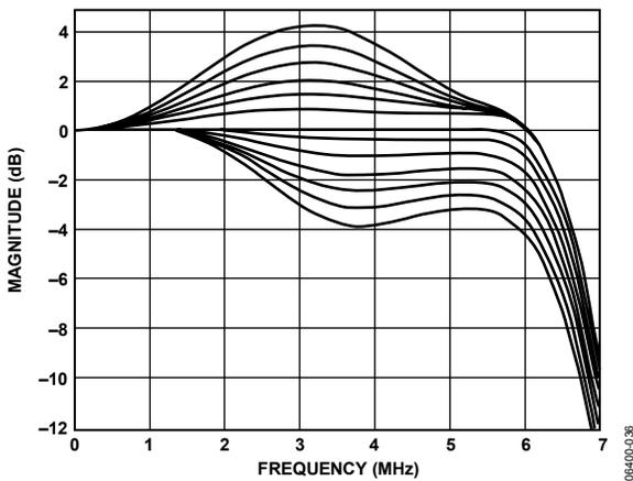
Figure 36. SD Luma SSAF Filter, Programmable Responses
