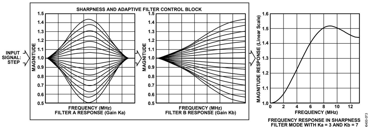
Figure 72. ED/HD Sharpness and Adaptive Filter Control Block
