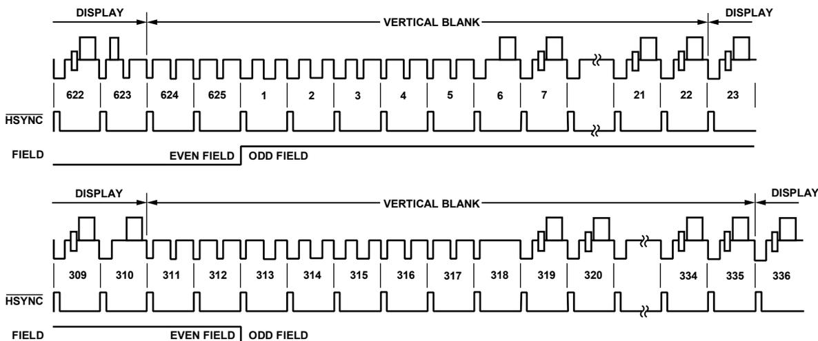
Figure 112. SD Timing Mode 3, PAL
