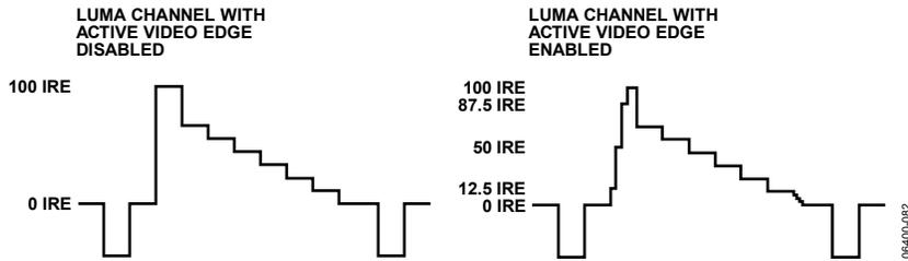
Figure 81. Example of Active Video Edge Functionality
