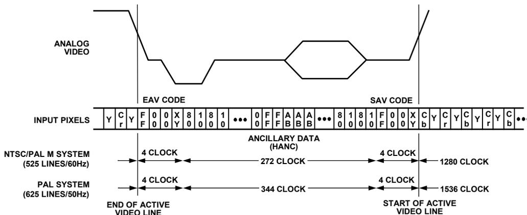
Figure 63. Square Pixel Mode EAV/SAV Embedded Timing
