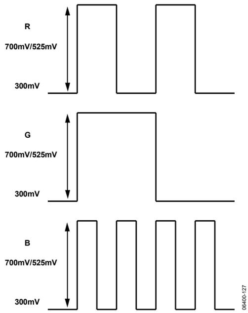
Figure 126. HD RGB Output Levels—RGB Sync Disabled
