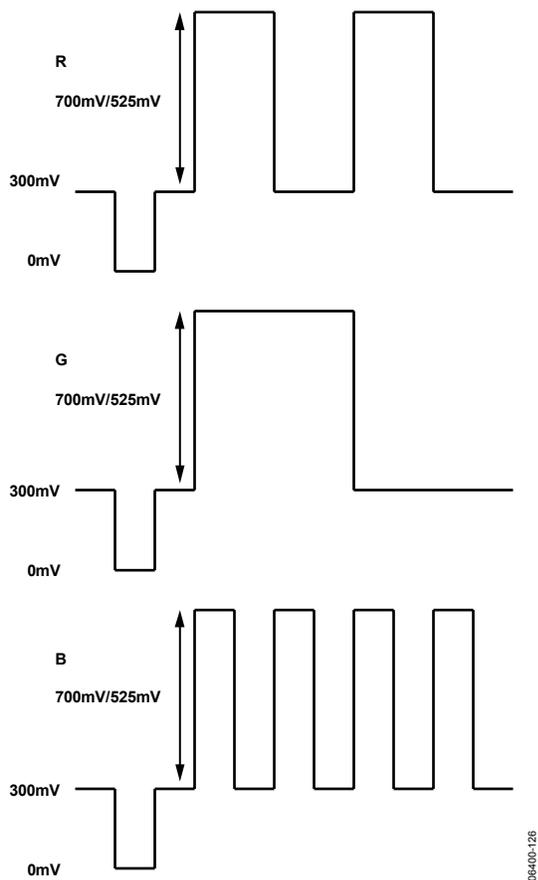
Figure 125. SD/ED RGB Output Levels—RGB Sync Enabled
