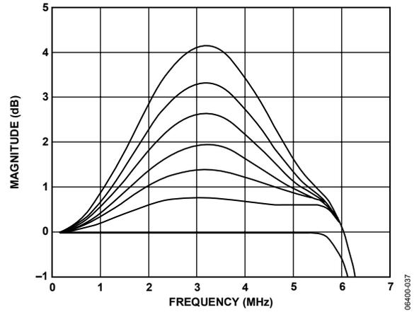
Figure 37. SD Luma SSAF Filter, Programmable Gain
