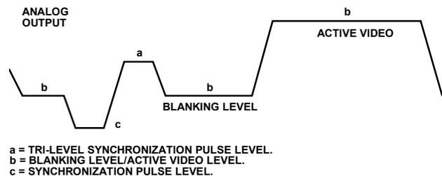
Figure 59. ED/HD Nonstandard Timing Mode Output Levels
