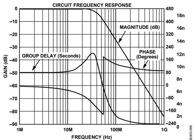
Figure 88. Output Filter Plot for ED, 8x Oversampling
