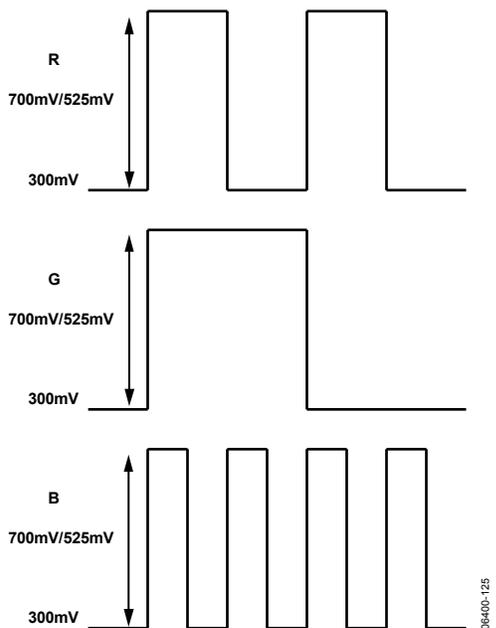
Figure 124. SD/ED RGB Output Levels—RGB Sync Disabled
