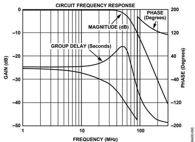
Figure 89. Output Filter Plot for HD, 4x Oversampling
