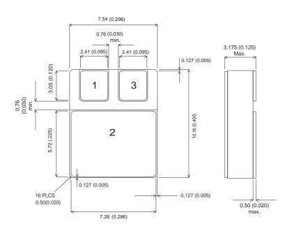
Bipolar NPN Device in a Hermetically sealed Ceramic Surface Mount
