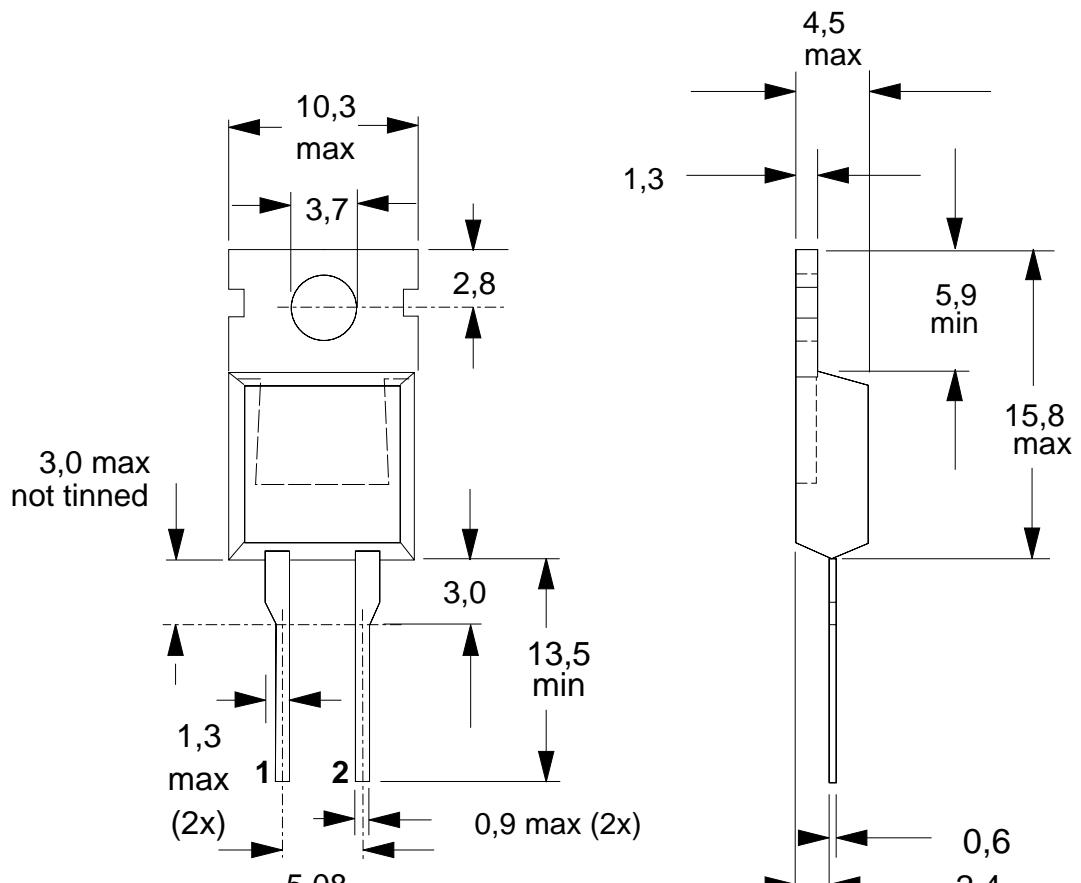
Fig.1. SOD59 (TO220AC). pin 1 connected to mounting base.
