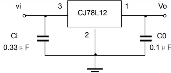
Note: Bypass capacitors are recommended for optimum stability and transient response and should be located as close as possible to the regulators.
