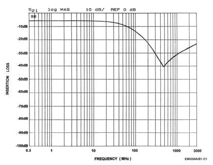
Figure 1. Microphone 1 Circuit (B1-C1) EMI Filter Performance
