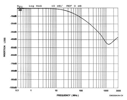
Figure 4. Speaker 2 Circuit (A4-C4) EMI Filter Performance
