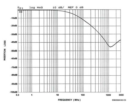
Figure 3. Speaker 1 Circuit (A3-C3) EMI Filter Performance
