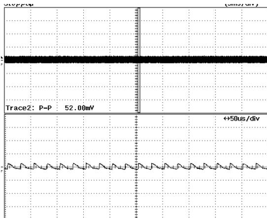
**Figure 19** – Ripple, 230 VAC, Full Load.
