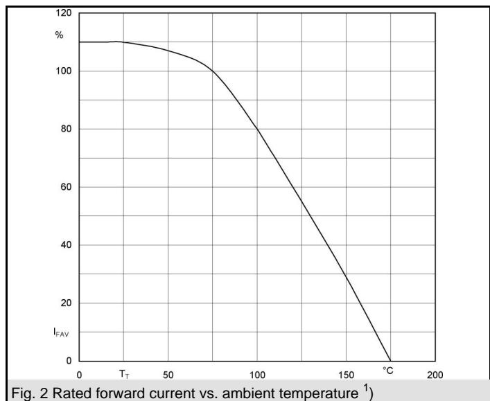
Fig. 2 Rated forward current vs. ambient temperature <sup>1)</sup>
