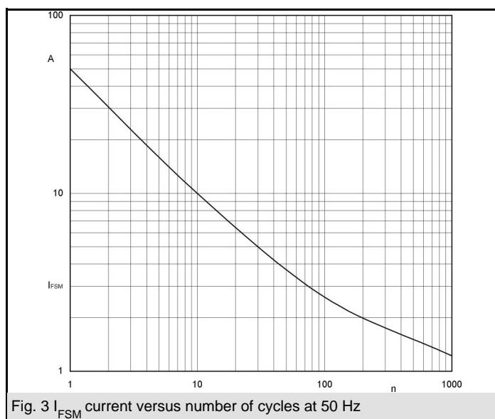
Fig. 3  $I_{FSM}$  current versus number of cycles at 50 Hz
