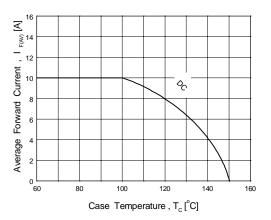
Figure 6. Forward Current Derating Curve
