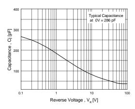
Figure 3. Typical Junction Capacitance
