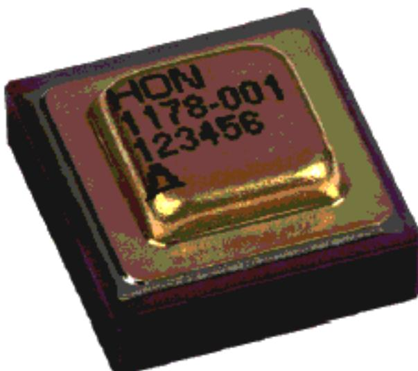
The device sensitivity (scale factor) is factory programmable from  $\pm 75^\circ/\text{sec}$  to  $\pm 300^\circ/\text{sec}$ . Output bandwidth is also factory programmable between 30 and 125 Hz.
