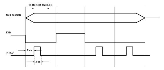
The encoder sends a pulse for every space or "0" that is sent on the TXD line. On a high to low transition of the TXD line, the generation of the pulse is delayed for 7 clock cycles of the 16XCLK before the pulse is set high for 3 clock cycles (or 3/16th of a bit time) and then subsequently pulled low.
