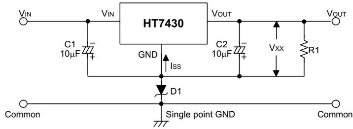
$$V_{OUT} = V_{XX} + V_{D1}$$
