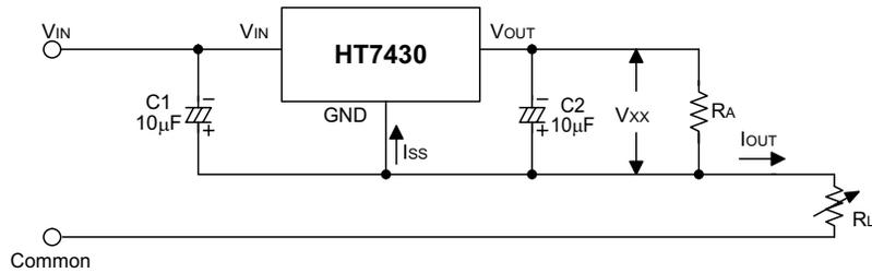
$$I_{OUT} = \frac{V_{XX}}{R_A} + I_{SS}$$
