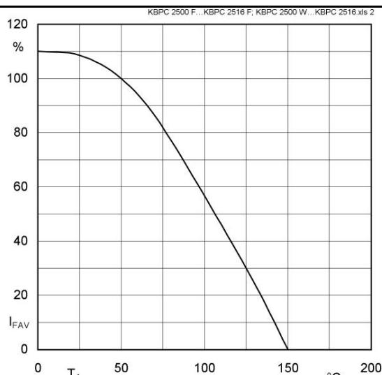
Fig. 2 : Rated forward current vs. ambient temperature
