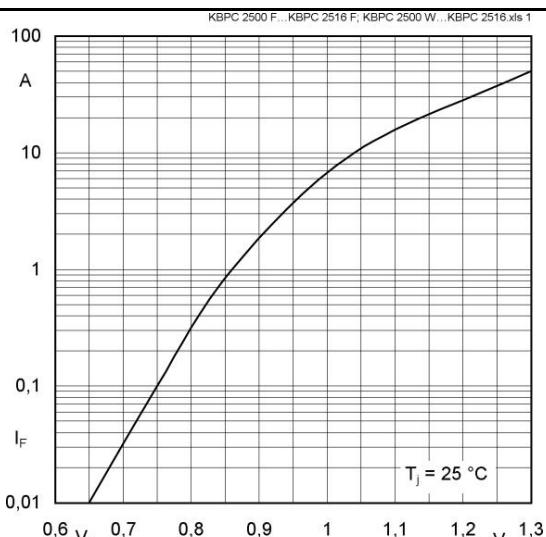
Fig. 1 : Forward characteristics (typical values)
