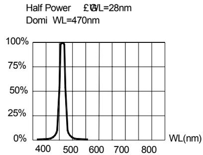
FIG.3 RELATIVE LUMINOUS FLUX VS. WAVELENGTH.
