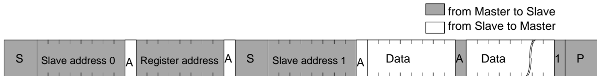
Figure 5.16 Master reads from M65863FP(slave) Register
